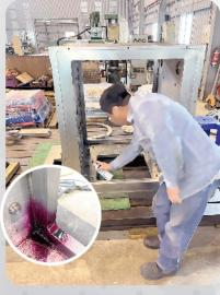
渗透探傷法Liquid Penetrant Testing / LPT
